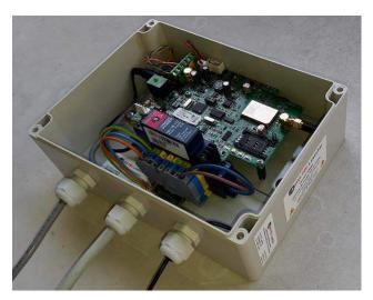
GSM Fixed Wireless Terminal that produces an analog phone line.
