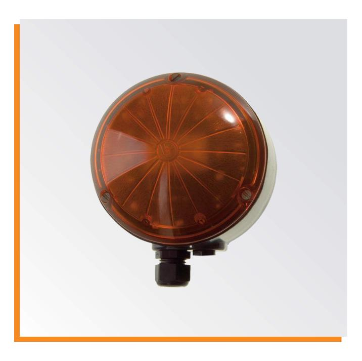
Phone signal Type DUO / SIP The DUO signals incoming calls both audibly and optically. The flash frequency and the signal tone can be set individually. The extensive settings can be configured via web-interface. The DUO / SIP is intended for wall mounting and is controlled by the integrated SIP telephone connecting relay. Power supply is via PoE or extern with 48V.
