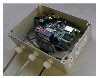
Simulation of an analogue telephone connection via 4G / LTE mobile network and the possibility of data transmission.
